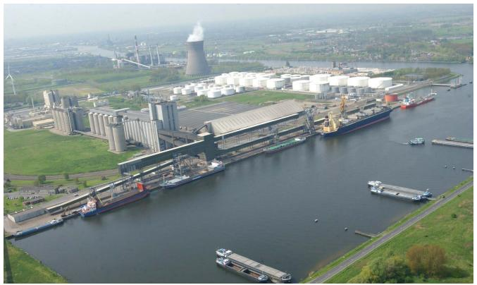
Rodenhuize Docks Area – Example of Co-location of Bio-refinery Components (AlcoBiofuel, Bioro, Cargill, Eletrabel, EuroSilo, Oiltanking) Source: Roland Verhe
