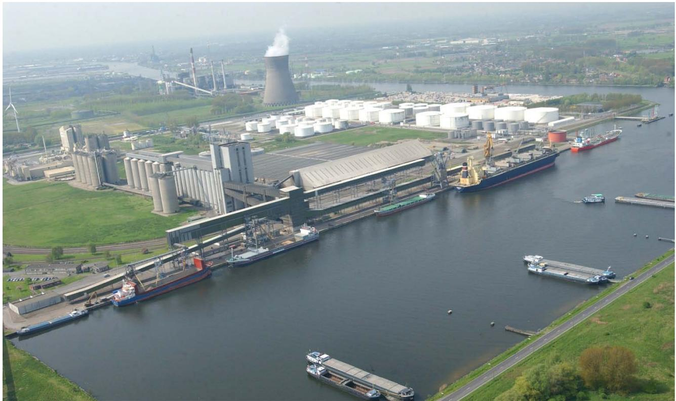
**Rodenhuize Docks Area – Example of Co-location of Bio-refinery Components (AlcoBiofuel, Bioro, Cargill, Eletrabel, EuroSilo, Oiltanking)**
